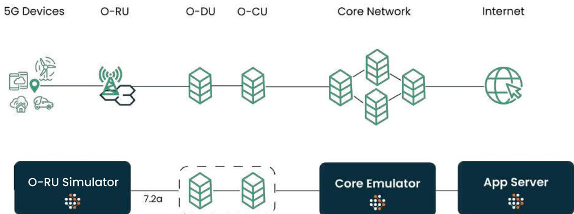
*Leverage wrap-around configuration for combined O-DU, O-CU testing.*
